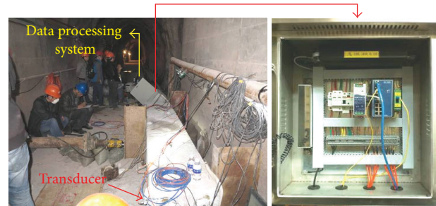
FIGURE 4: Microseismic monitoring system network.
