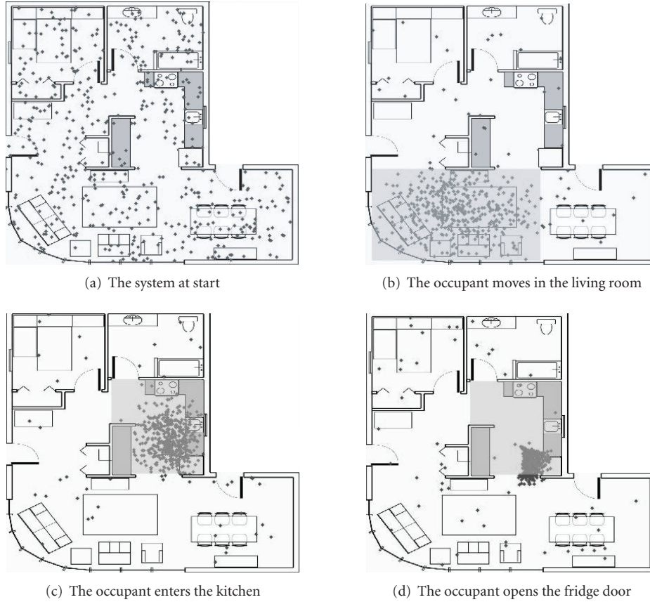
FIGURE 1: The localization system in a real condition situation. The points show the particle cloud. The shaded areas indicate where the occupant is likely to be present.
