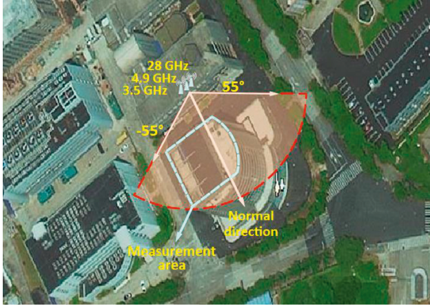
FIGURE 2: Multiband O2I channel measurement scenario.
