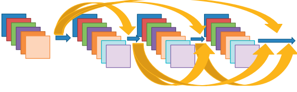
FIGURE 1: The dense connection mechanism of the DenseNet.
