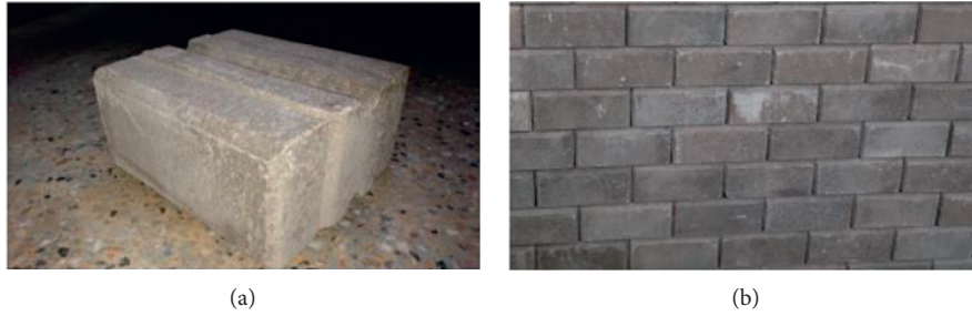
FIGURE 1: (a) Hydraform block. (b) Assemblage of dry-stacking Hydraform blocks.
