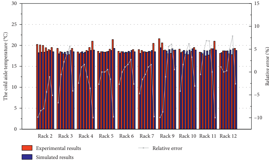
FIGURE 3: Temperature comparison of experimental and simulation results in cold aisles.
