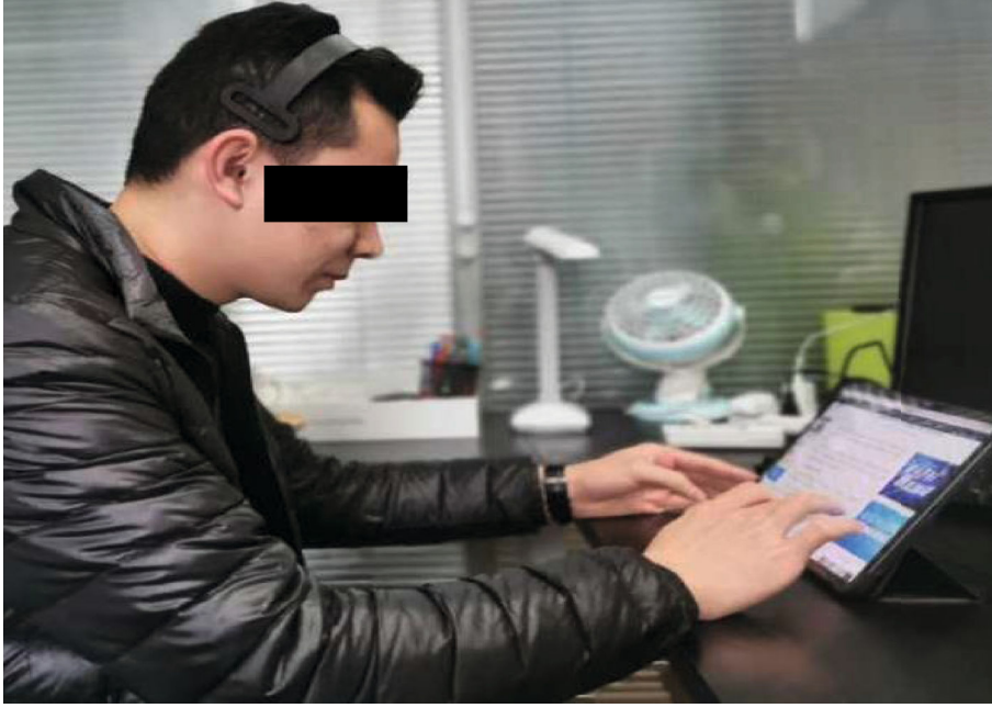
FIGURE 3: EEG measurement process. The participant was being tested while using an iPad.
