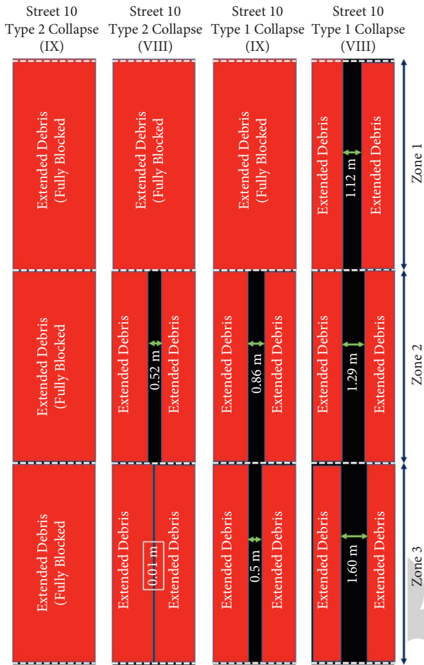
FIGURE 11: Representative figure for the obstructed zones of street number 10.
