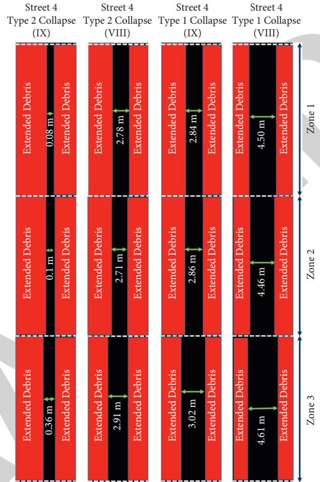
FIGURE 10: Representative figure for the obstructed zones of street number 4.
