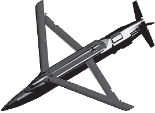
FIGURE 1: Sketch of small diameter bomb with diamond back wing.
