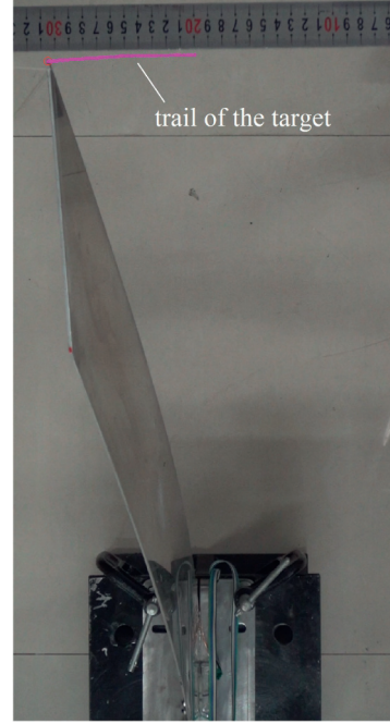
FIGURE 7: Target tracking in image plane for the wind-off experiment.
