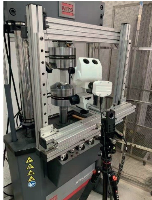
FIGURE 2: MTS fatigue testing machine system.
