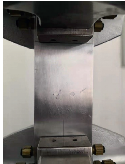
FIGURE 3: Test diagram of two-hole plate specimen.
