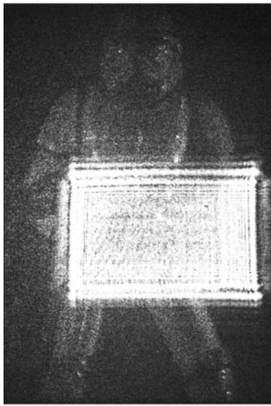
FIGURE 14: Optical reconstruction of holographic data with SLM: reconstruction of intensity hologram.
