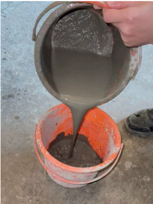
FIGURE 9: Flow pattern of filling slurry.
