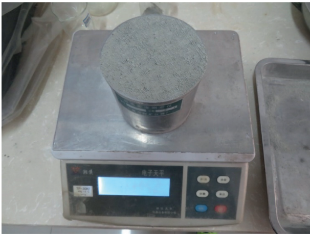
FIGURE 2: Bulk density determination process.
