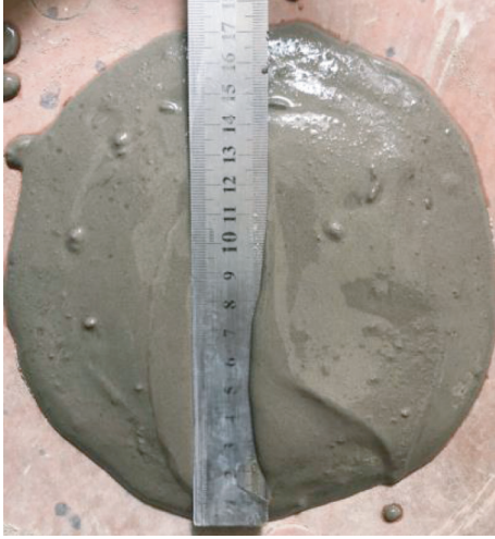
FIGURE 3: The fluidity test of Aeolian sand-like paste [12].
