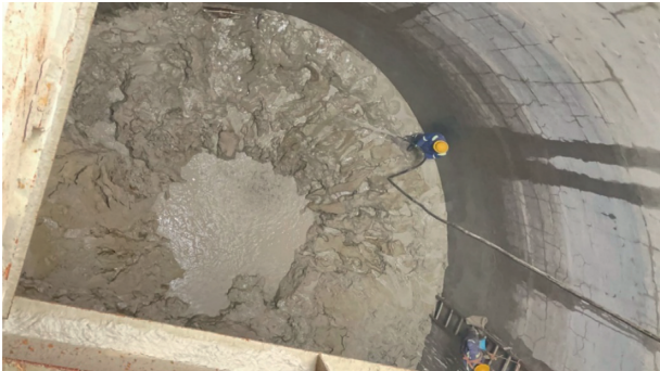
FIGURE 11: Deposition and consolidation of tailings.
