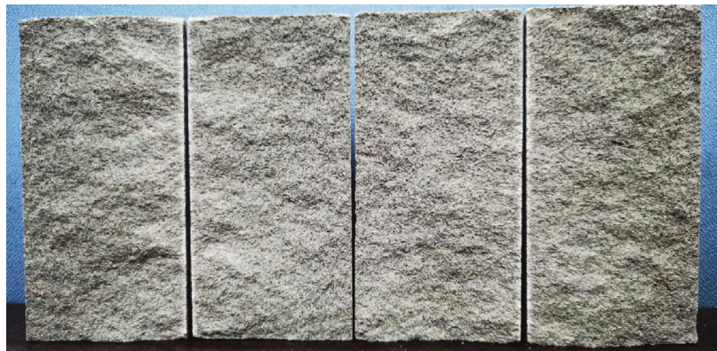
(c) Fracture surface after the Brazilian testing
