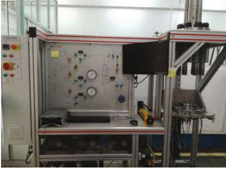
FIGURE 3: Triaxial multifield coupling test system.
