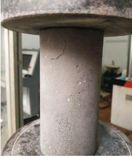
FIGURE 4: Uniaxial compressive strength test.
