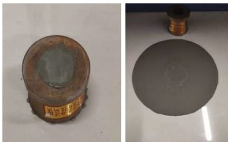
FIGURE 3: Cement fluidity test.
