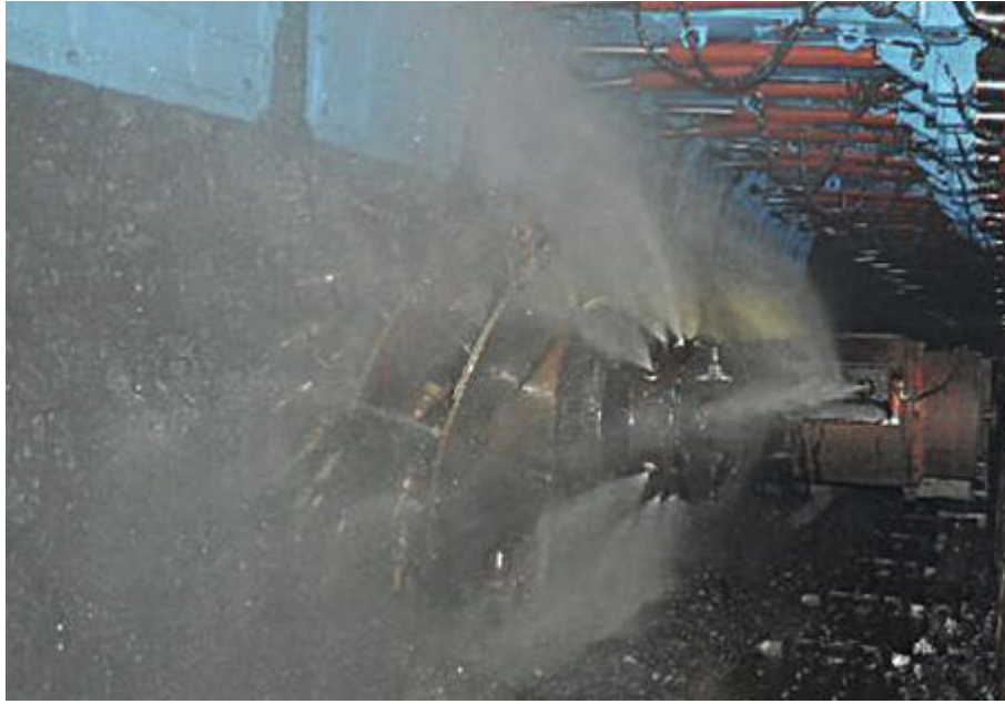
FIGURE 10: Field application diagram of negative dust collecting device in coal mining operation.
