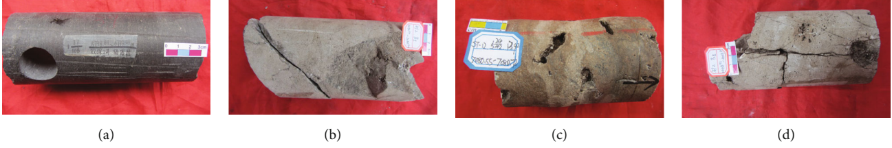
FIGURE 1: Core sampling of the petrophysical experiment: (a) reservoir with matrix pores, (b) reservoir with matrix pores and fractures, (c) reservoir with matrix pores and vugs, and (d) reservoir with matrix pores, fractures, and vugs.
