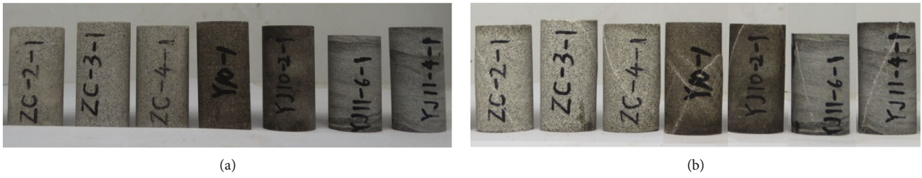
FIGURE 2: Tight sandstone cores. (a) Initial state. (b) After failure.
