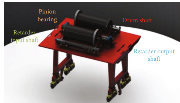
FIGURE 13: The component-system structure of the crane trolley.
