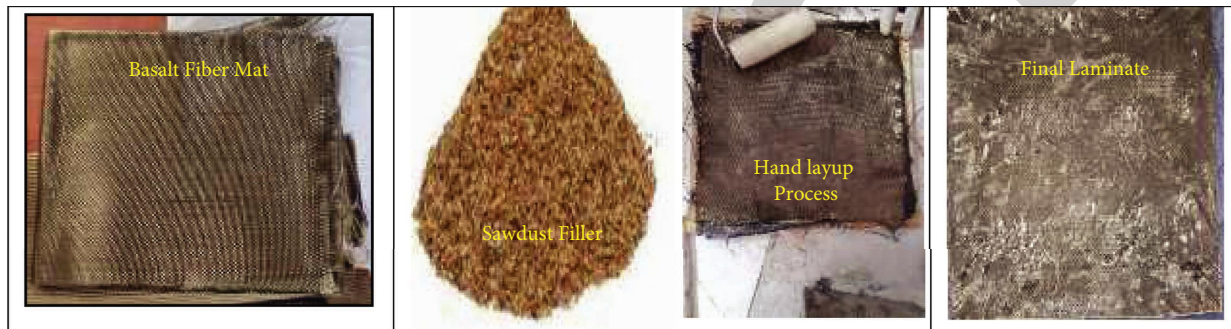
FIGURE 2: Fabrication process of basalt fiber composite.
