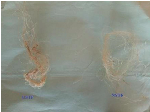
FIGURE 2: Extracted fiber with untreated and NaOH treated.
