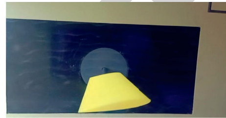
FIGURE 22: Wind tunnel testing of 3d printed airfoil.
