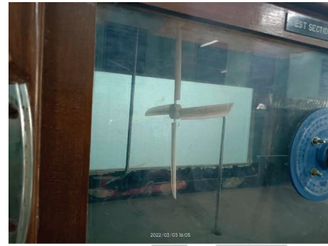
FIGURE 7: HH02 rotor model in the wind tunnel.
