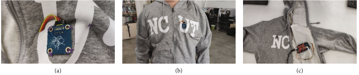
FIGURE 2: LoRa wearable integrated sensors: (a) the position of a LoRa node on clothing; (b) person wearing the clothing; (c) the clothing inside view.
