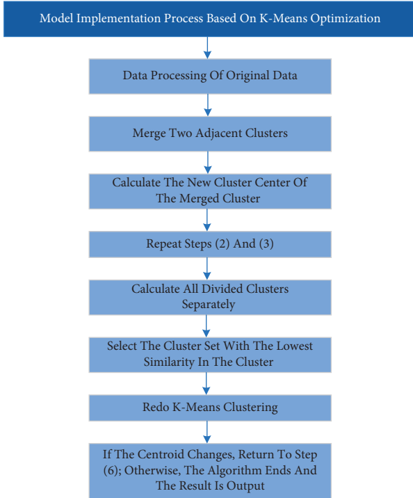
FIGURE 5: Optimization process based on K-Means.
