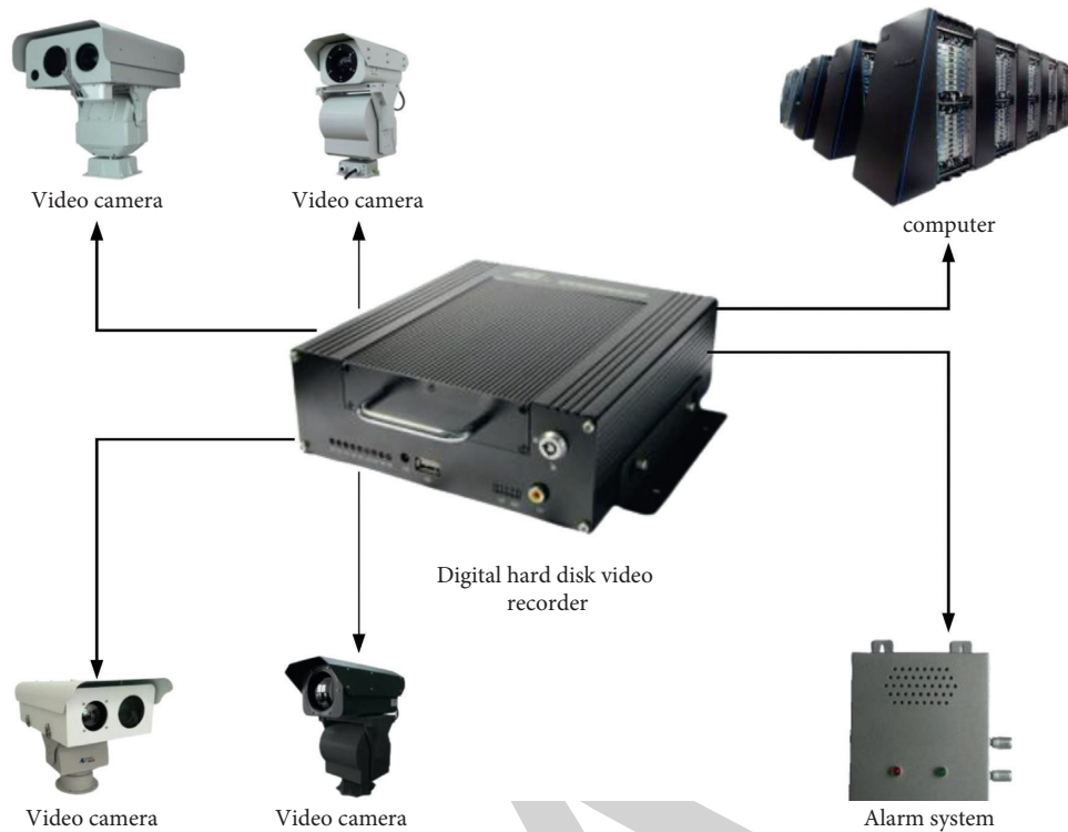
FIGURE 1: Train image monitoring system structure.
