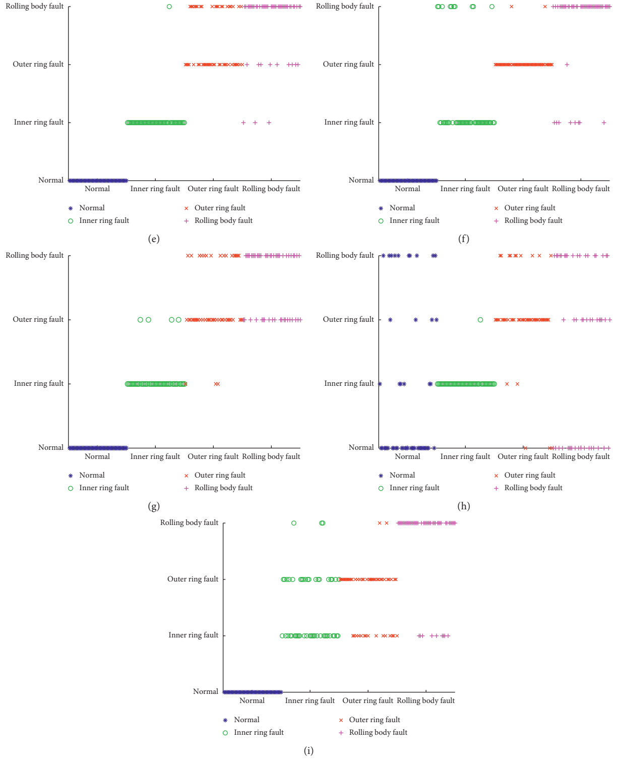
FIGURE 10: The characteristic classification results of the center frequency of each IMF. (a) IMF1. (b) IMF2. (c) IMF3. (d) IMF4. (e) IMF5. (f) IMF6 (g). IMF7 (h). IMF8. (i) IMF9.
