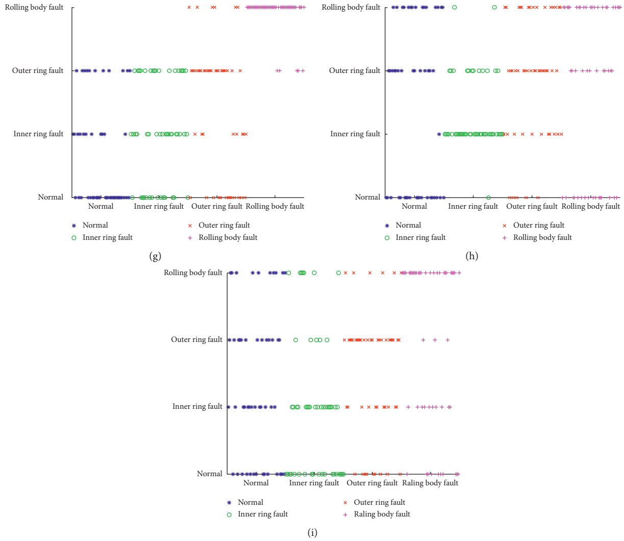
FIGURE 11: The characteristic classification results of the envelope entropy of each IMF. (a) IMF1. (b) IMF2. (c) IMF3. (d) IMF4. (e) IMF5. (f) IMF6 (g). IMF7 (h). IMF8. (i) IMF9.
