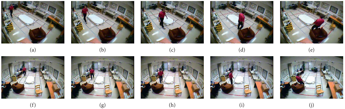
FIGURE 5: The position change of the linear trajectory of the same target in different perspectives (from top to bottom are the perspectives 1 and 2 and from left to right are the frames 22, 33, 44, 55, and 66).
