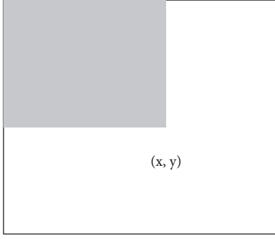
FIGURE 1: Integral image value at the point (x, y) .
