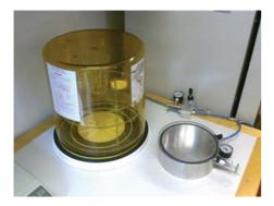
FIGURE 1: Degassing chambers used to degas the samples.
