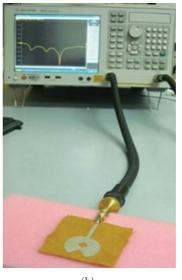
Figure 3: Snapshot of ( $|S_{11}|$ ) measurement environment of both antenna prototypes using (a) copper conducting tape and (b) Shieldit conducting fabric.
