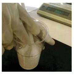
FIGURE 2: Vigorous mixing of PDMS ceramic powder with PDMS mixture.
