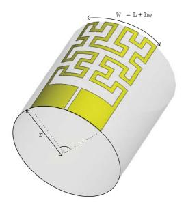
FIGURE 3: Geometry of the flexible Hilbert-curve loop antenna and radius of its curvature.
