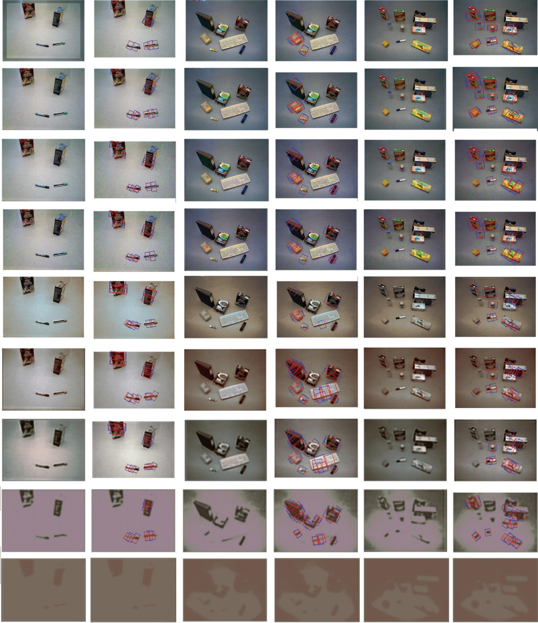
FIGURE 9: The first line is the result of the grasp detection of the original image, and the lines below are the results under the compression ratio of 16.29%, 4.07%, 0.99%, 0.5%, 0.13%, 0.05%, 0.04%, and 0.03%. From top to bottom, the loss of pictures due to compression gradually increases, which slowly affects the bounding box results of grasp detection.
