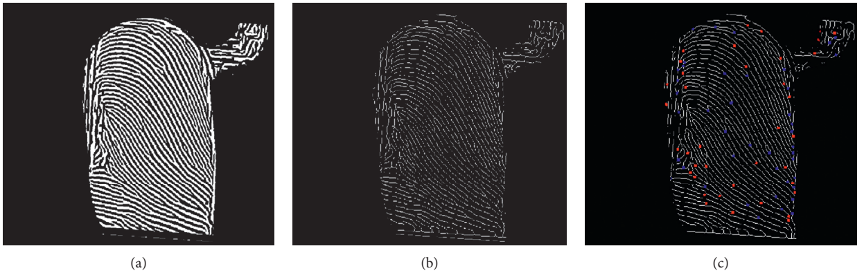
FIGURE 6: Applying edge thinning operations to an enhanced image: (a) binary segmentation, (b) nonmaximal suppression, and (c) minutiae extraction.
