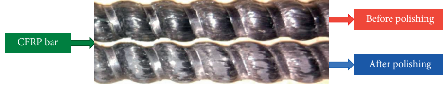
FIGURE 3: Shape of the CFRP bar.
