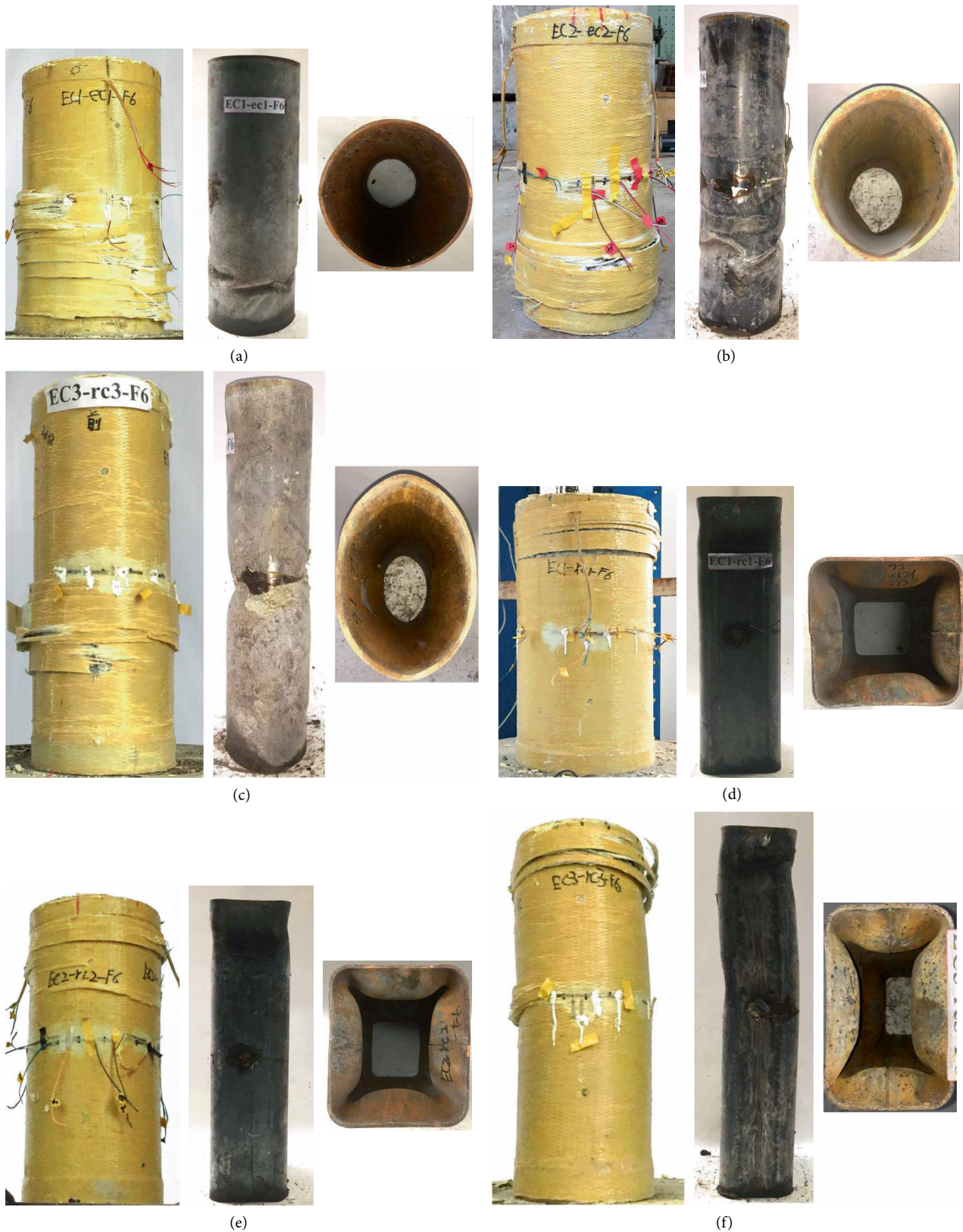
FIGURE 7: Typical specimens after test. (a) EC1-ec1-F6. (b) EC2-ec2-F6. (c) EC3-ec3-F6. (d) EC1-rc1-F6. (e) EC2-rc2-F6. (f) EC3-rc3-F6.
