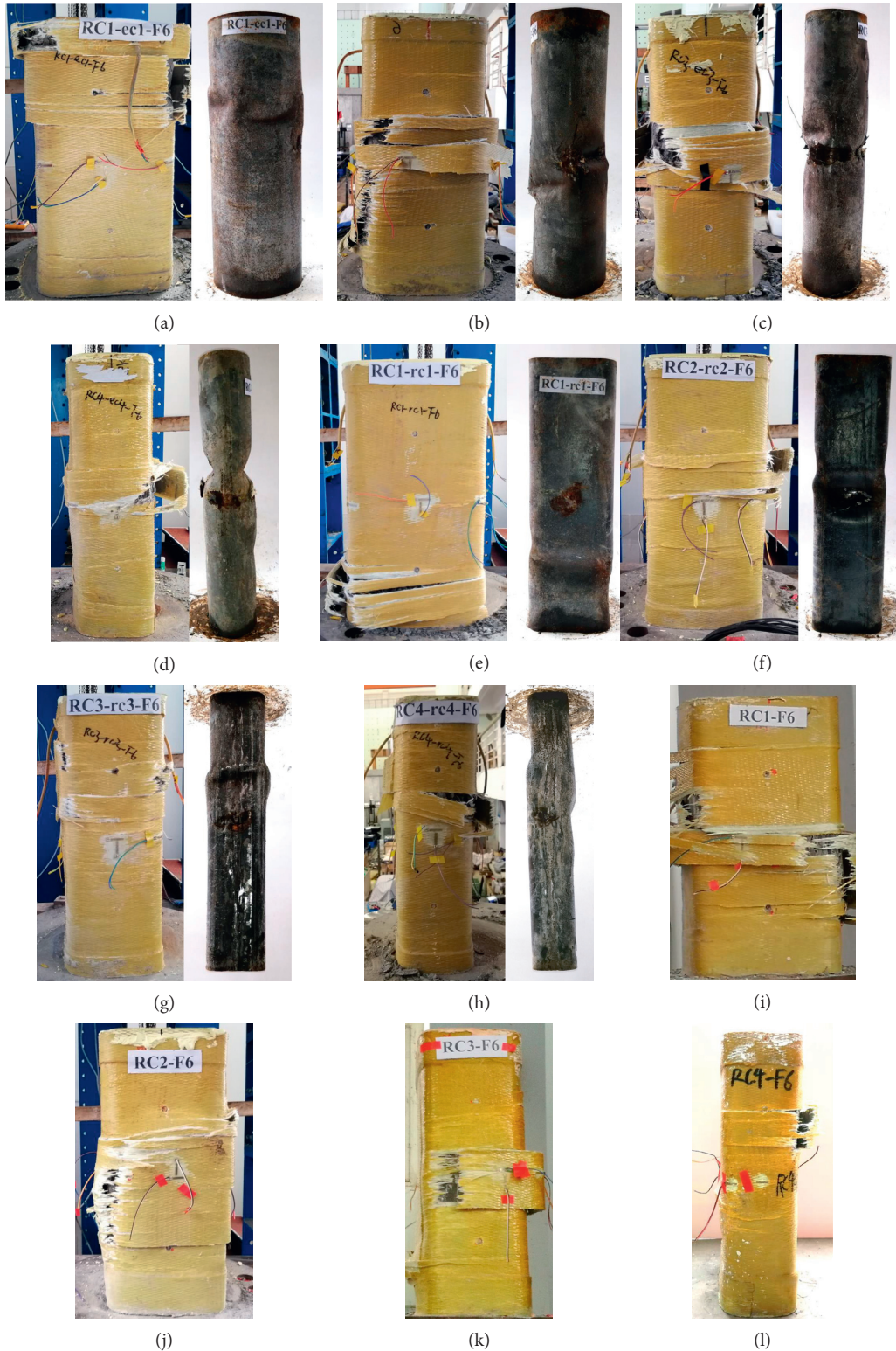
FIGURE 6: Typical failed specimens after test. (a) RC1-ec1-F6, (b) RC2-ec2-F6, (c) RC3-ec3-F6, (d) RC4-ec4-F6, (e) RC1-rc1-F6, (f) RC2-rc2-F6, (g) RC3-rc3-F6, (h) RC4-rc4-F6, (i) RC1-F6, (j) RC2-F6, (k) RC3-F6, and (l) RC4-F6.
