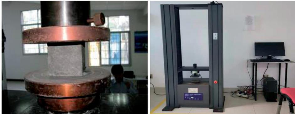
FIGURE 6: Laboratory UCS test.
