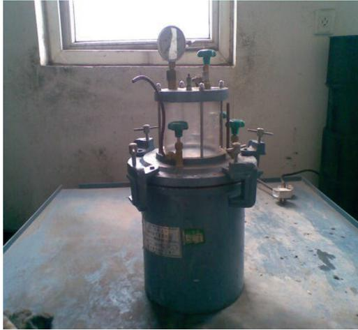
FIGURE 2: The gas content test.
