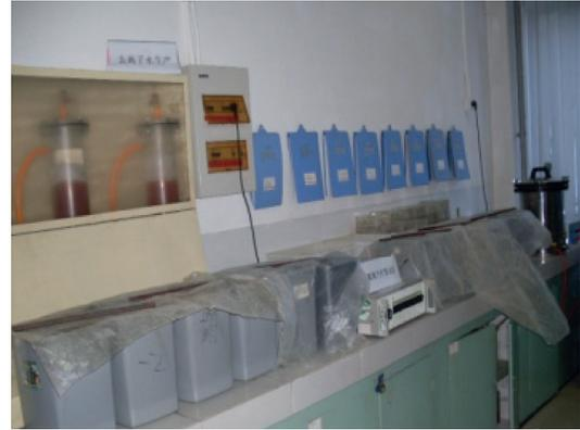
FIGURE 3: The electric flux test.
