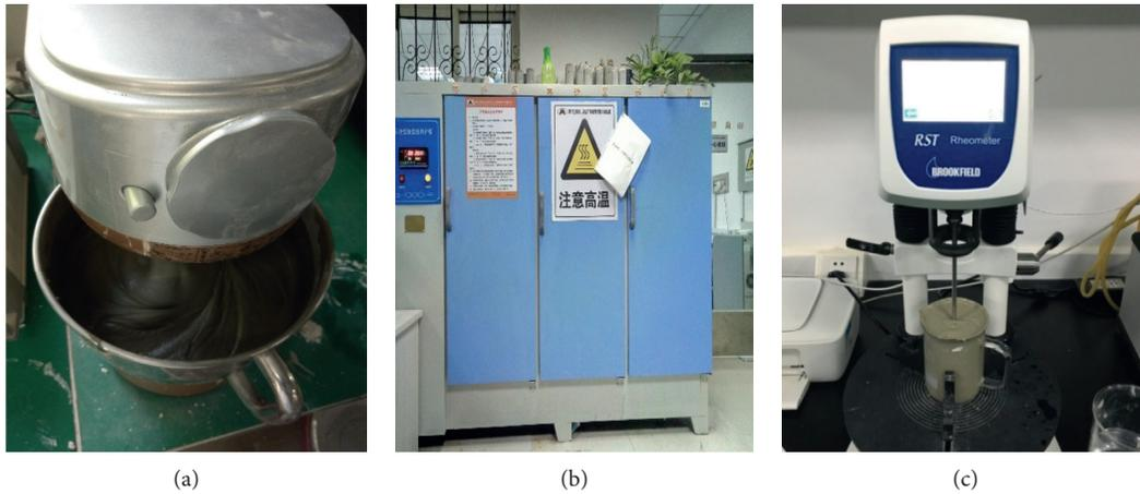
FIGURE 6: The preparation stages of CPB samples: (a) mixing, (b) curing, and (c) testing.
