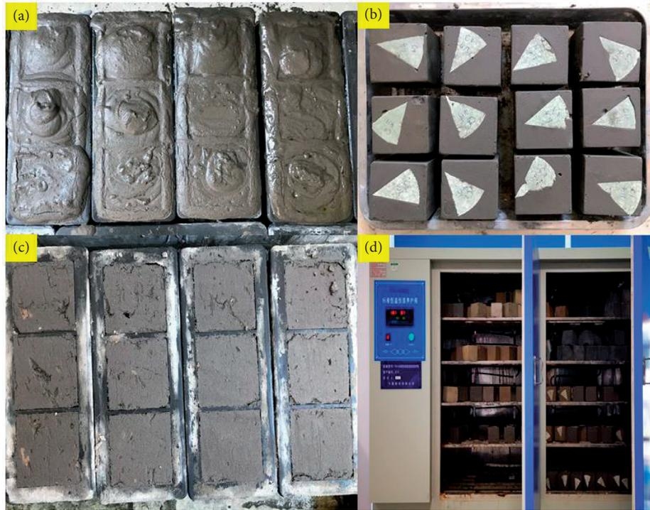
FIGURE 5: CPB specimens preparation and curing process.
