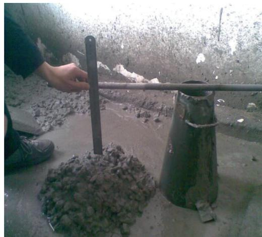
FIGURE 1: The slump test.
