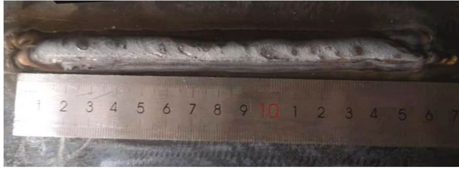
FIGURE 4: The macro morphology of additively manufactured ER50-6.
