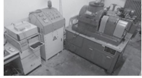
FIGURE 1: Bearing fatigue life test bench.
