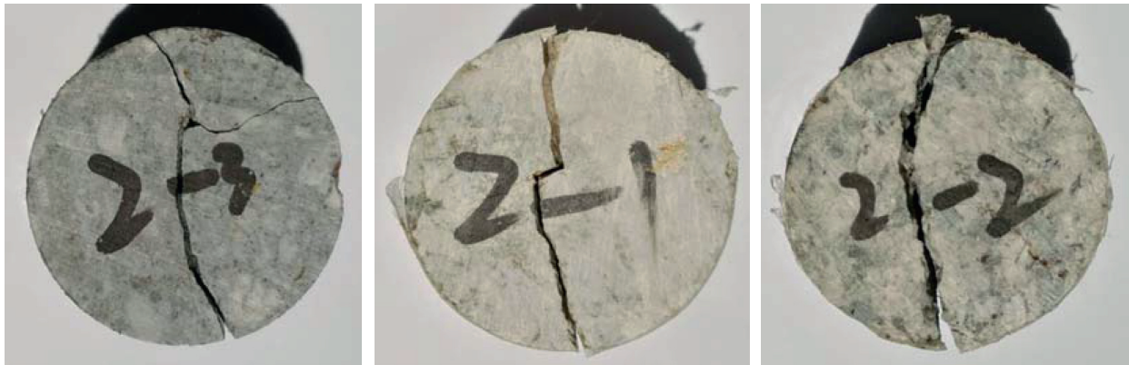
FIGURE 4: Brazil disk split test with granite specimens.
