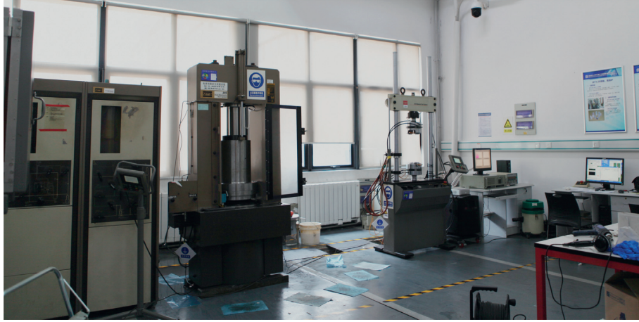
FIGURE 3: MTS815.02 electrohydraulic servo rock mechanics test system.
