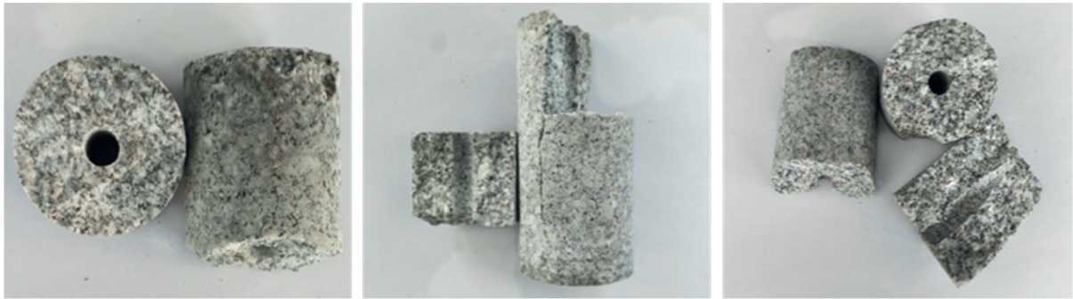
FIGURE 11: Fracture failure morphology of granite specimens with a vertical hole under different impact pressures of equal-amplitude impact.
