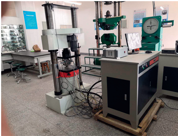
FIGURE 6: YAW-2000 computer-controlled automatic pressure testing machine.
