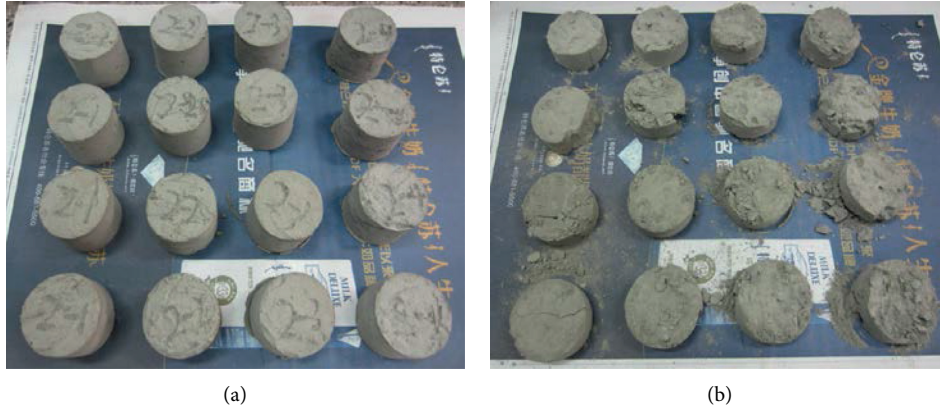
FIGURE 3: Shear test photos: (a) prepared specimens; (b) specimens destroyed.
