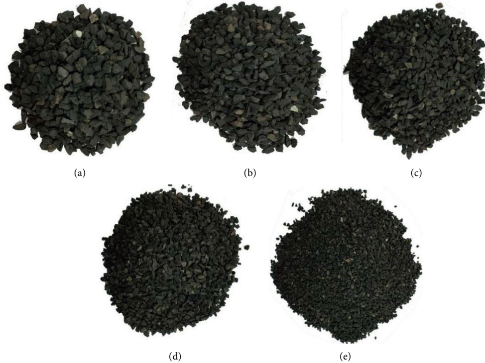
FIGURE 1: Classification of particle size: (a) 20.0~25.0 mm. (b) 15.0~20.0 mm. (c) 10.0~15.0 mm. (d) 5.0~10.0 mm. (e) 2.5~5.0 mm.
