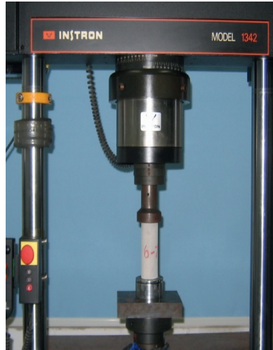
FIGURE 5: Creep experiment of the filling body.
