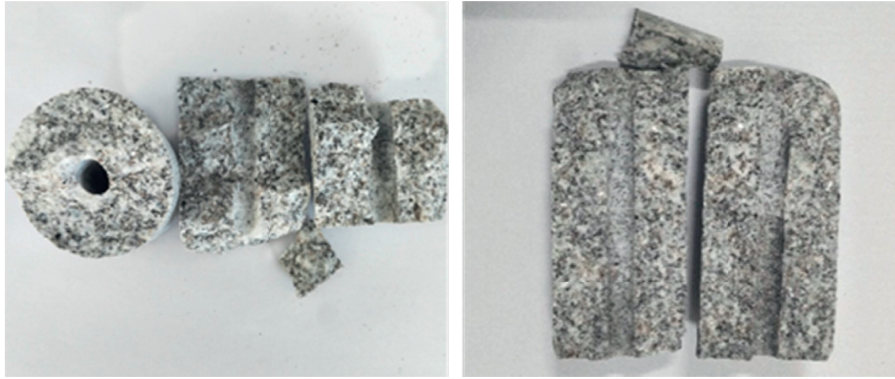
FIGURE 12: Fracture failure morphology of the granite specimen with a vertical hole under different impact pressures with unequal-amplitude impact.
