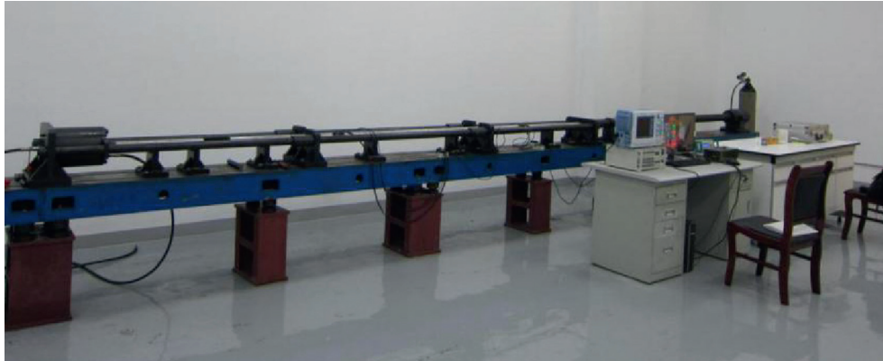
FIGURE 4: SHPB test device.
