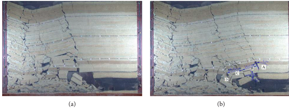
FIGURE 15: Model overview before and after key stratum breaking. (a) Before key stratum breaking and (b) after key stratum breaking.
