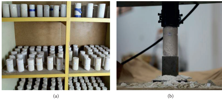
FIGURE 5: Strength test of similar materials [1]. (a) Sample of similar material and (b) strength test process.
