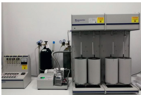
FIGURE 3: ASAP 2460 multistation specific surface and porosity analyzer.
