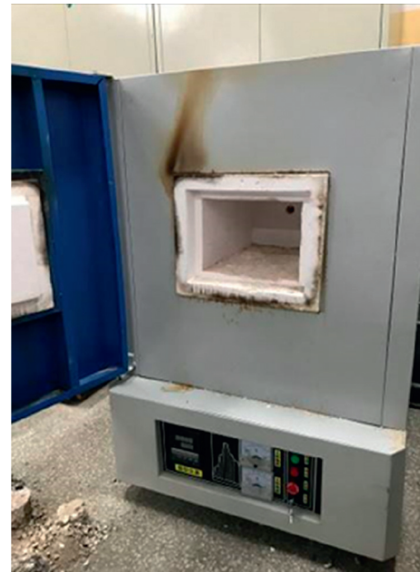
FIGURE 4: XH7L chamber-type electric resistance furnace.
