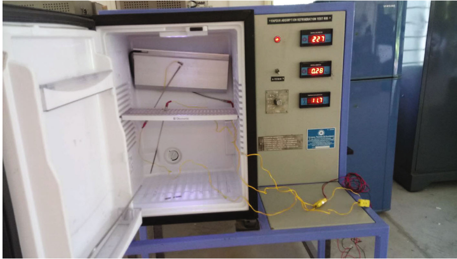
FIGURE 5: Experimental setup of AC VAR.
