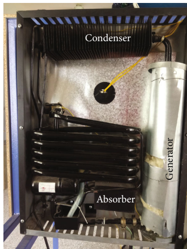
FIGURE 2: Components of the VAR system.
