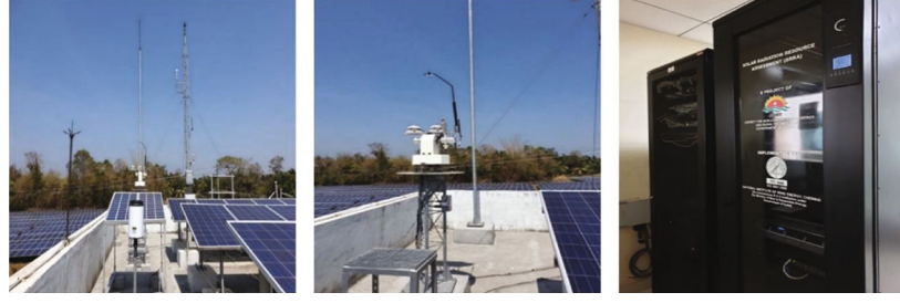
FIGURE 2: Dedicated SRRA station at the site and central data server for the real-time collection of the data.
