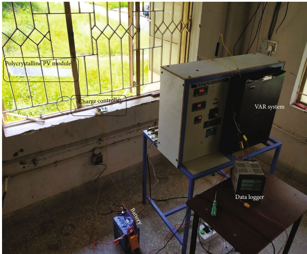
FIGURE 6: Experimental setup of solar PV-powered VAR.
