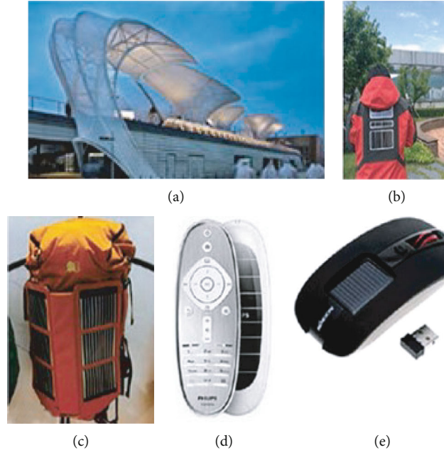
FIGURE 7: Examples of applications of OPVs: (a) building-integrated photovoltaics, (b) jacket with an incorporated OPV module, (c) backpack, (d) remote control, and (e) solar computer mouse [99].
