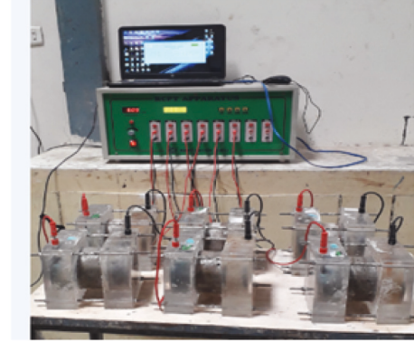
FIGURE 4: Test setup for RCPT test.
