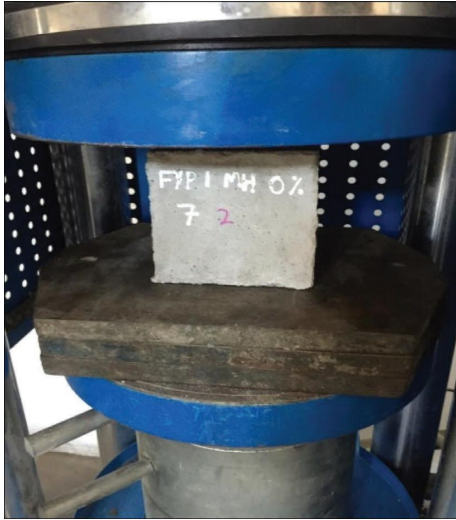
FIGURE 4: Compression test machine.
