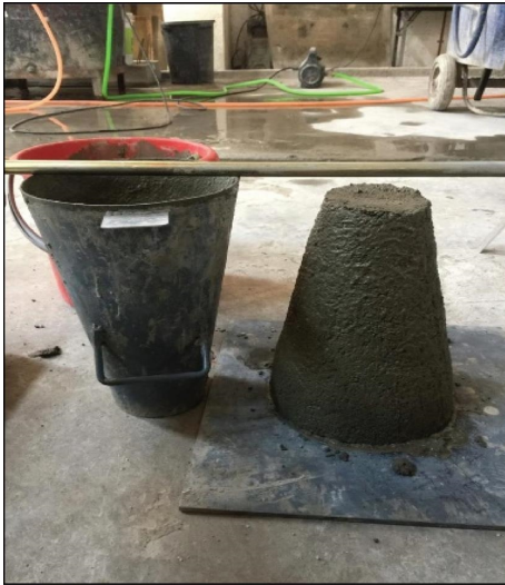
FIGURE 2: Slump test.
