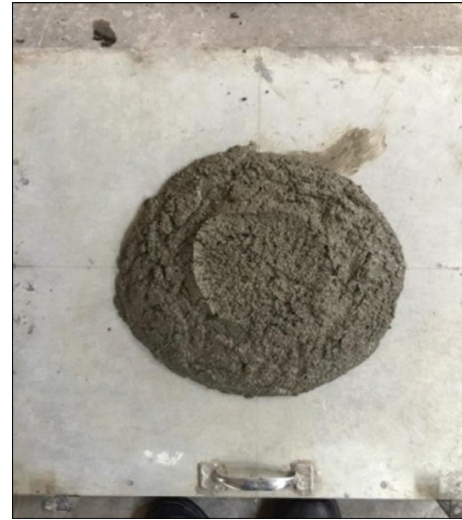
FIGURE 3: Flow table test.
