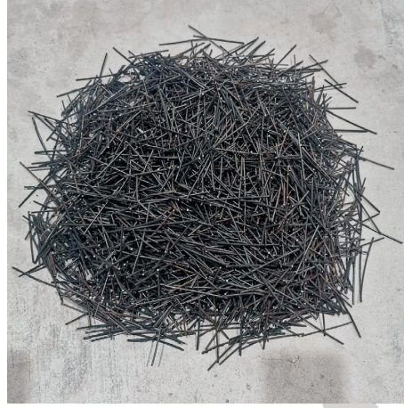
FIGURE 1: Recycled steel fibers.
