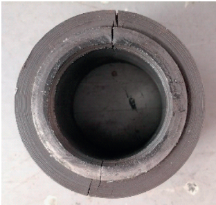
FIGURE 5: Crack damage of roller.
