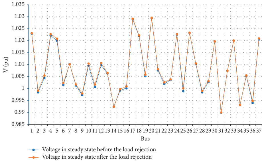
FIGURE 10: Compare the voltage when generator outage and after load shedding according to the proposed method.
