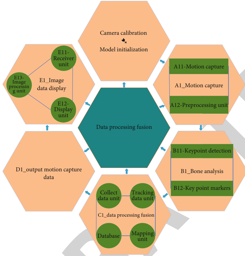
FIGURE 2: Motion capture system operation flow.
