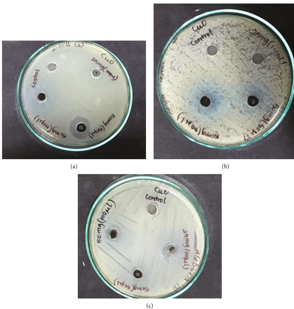
FIGURE 1: Bactericidal activity of CuO-NPs: (a) E. coli ; (b) S. aureus ; (c) K. pneumoniae .
