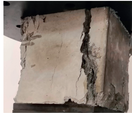
FIGURE 4: Macroscopic cracks on the outer surface of the concrete.
