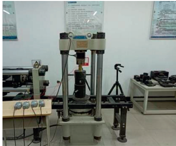
FIGURE 2: Site of the acoustic emission monitoring experiment under uniaxial compression.
