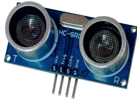
FIGURE 3: Ultrasonic sensor.
