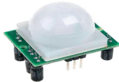
FIGURE 4: Passive infrared sensor.
