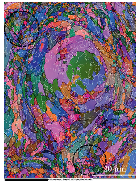
FIGURE 3: Euler angle EBSD patterns of the cross section of an Al 6061 particle in the cold-sprayed coating [18].
