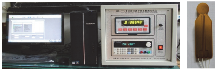
FIGURE 11: DRE-III heat conductivity coefficient tester and measuring probe.
