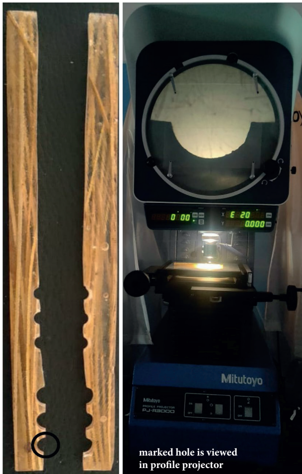
FIGURE 6: Periphery of the drilled hole is viewed using profile projector.
