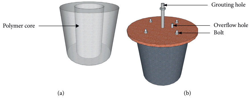
FIGURE 1: (a) Test piece schematic. (b) Steel cylinder.
