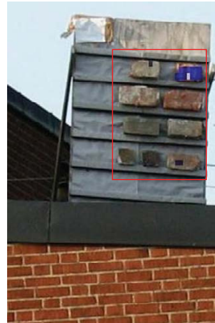
FIGURE 2: The brick samples measured, with an analysis superimposed. It was possible to delineate one of the brick samples by correlating all spectra with one spectrum on this particular brick. The white spot corresponds to the chosen reference spectrum and the blue points display the correlation coefficient value. Values below a certain threshold value have not been displayed. The scan was performed over all the bricks and contained 26 \times 22 points, as indicated by the red frame. As can be seen, the points on the particular brick have high correlation values and only a few points in the rest of the scan have values above the threshold.
