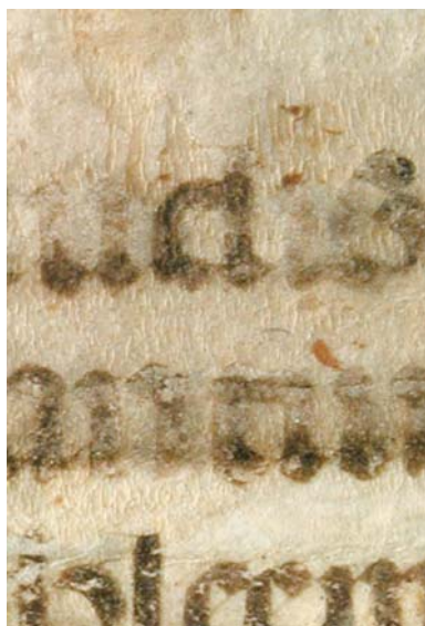
FIGURE 4: Macro photograph of the sample of historical parchment. Traces of water damage are visible.
