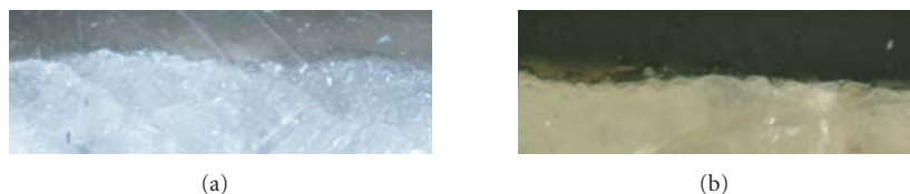
FIGURE 8: Stratigraphies of the treated parts on sample R. (a) 15 ns ( F_L = 1.4 \text{ J/cm}^2 ), (b) 90 \mu\text{s} ( F_L = 9.0 \text{ J/cm}^2 ) (20 \times magnification).
