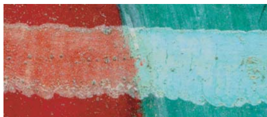
FIGURE 5: Result of ablation of varnish (Winsor & Newton Matt Varnish) over different underlying paint layers using the same fluence ( 1.7 \text{ J/cm}^2 ).
