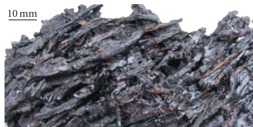
FIGURE 3: Particular of the manufacture surface. The presence of consolidant, round off the surface, makes it shiny.
