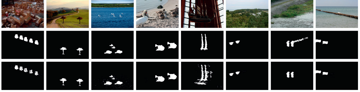
FIGURE 12: Copy-move forgery detection results for the JPEG. Top to bottom: test images from dataset, ground-truth forged regions, and forged regions detected by the proposed algorithm. Left to right, the quality factor is 20, 30, 40, 50, 60, 70, 80, and 90.
