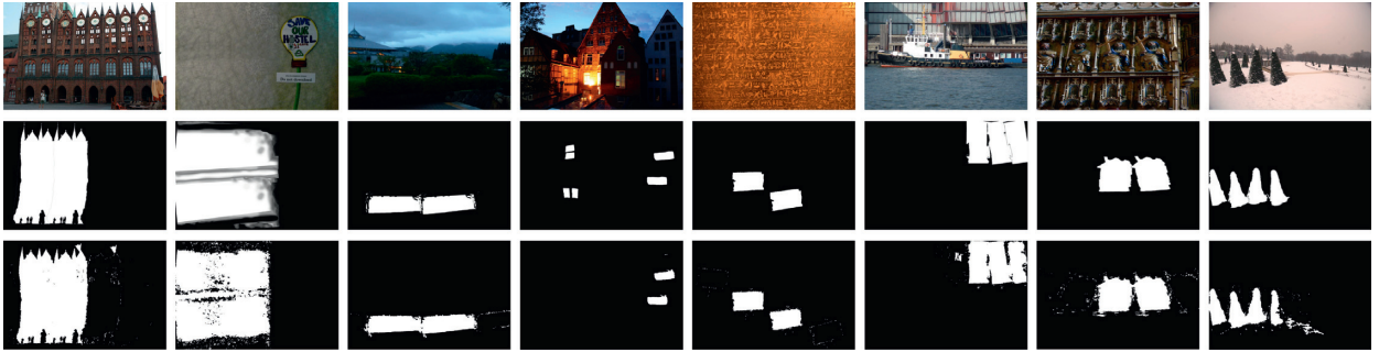
FIGURE 10: Copy-move forgery detection results for the rotation. Top to bottom: test images from dataset, ground-truth forged regions, and forged regions detected by the proposed algorithm. Left to right, the angle of rotation is 2^\circ , 4^\circ , 4^\circ , 6^\circ , 6^\circ , 8^\circ , 8^\circ , and 10^\circ .
