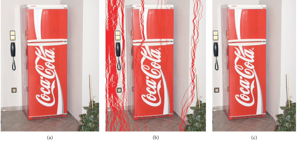
FIGURE 1: An image resized by seam carving. (a) An original image. (b) The image with vertical seams. (c) The seam-carved image.
