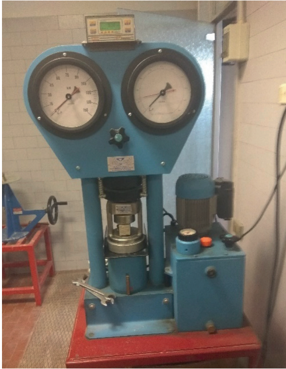
FIGURE 5: Compressive test on cubic sample.
