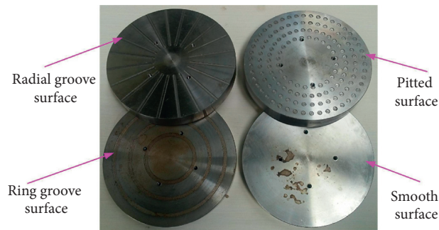
FIGURE 7: Drive plate with different surface topography.
