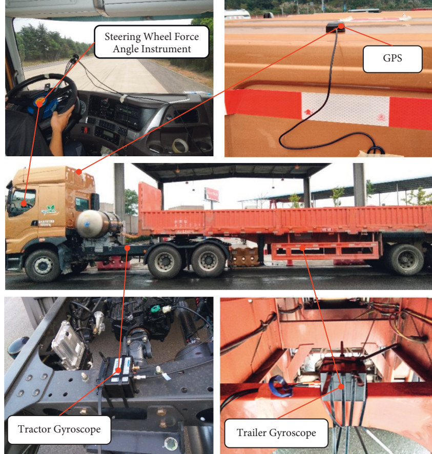
FIGURE 4: The installation position of test equipment.
