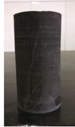
FIGURE 6: The failed specimen in the uniaxial compression tests.
