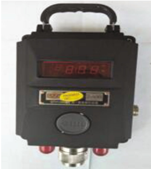
FIGURE 2: CO volume concentration sensor.
