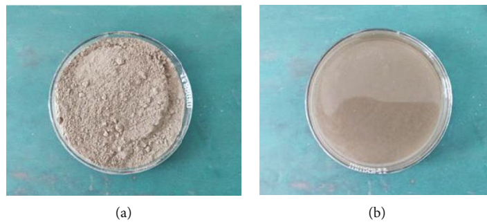
FIGURE 6: Injection material. (a) Fly ash and (b) injection slurry.
