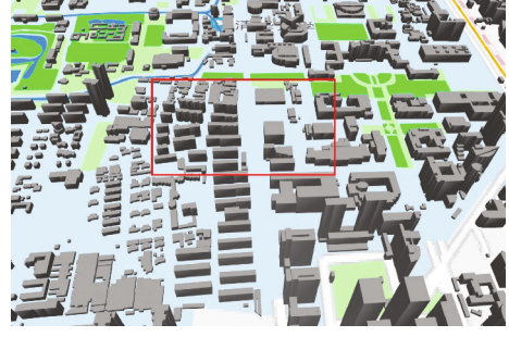
FIGURE 2: The established three-dimensional geographic model of Tsinghua University (grey, green, and blue objects, respectively, represent buildings, vegetation, and rivers).
