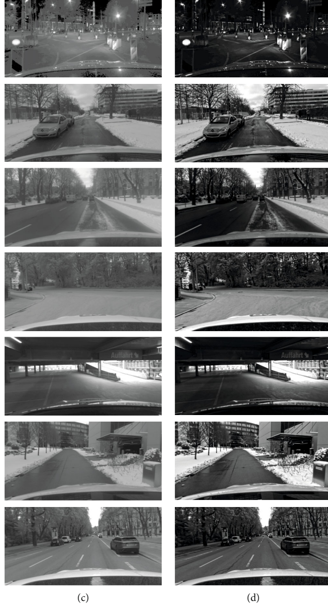
FIGURE 8: Results of the histogram equalization, adaptive gamma correction, and low-light image enhancement schemes. (a) The original image. (b) The results of histogram equalization. (c) The outcome of adaptive gamma correction. (d) The results of low-light image enhancement we used.
