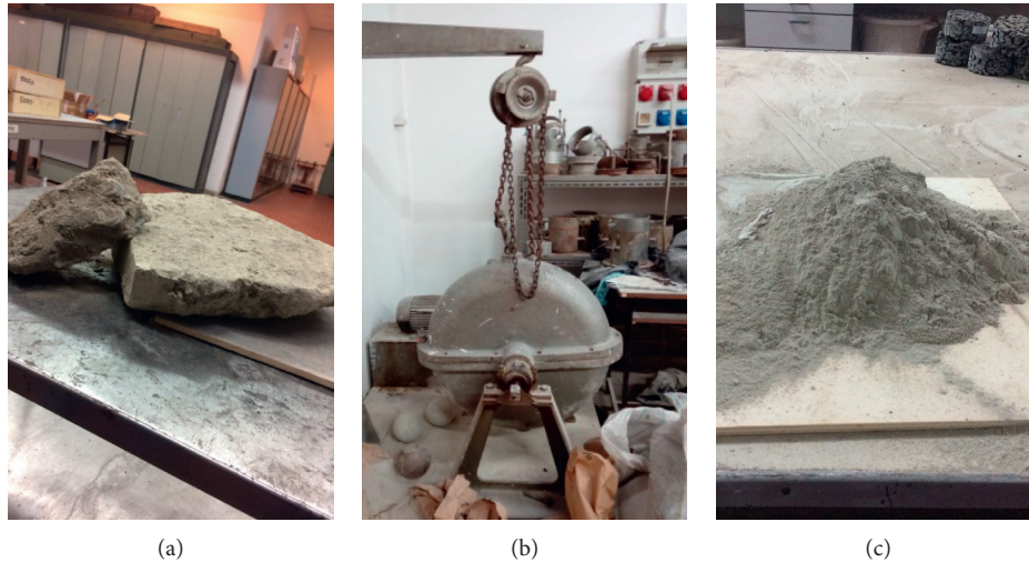
FIGURE 2: Jet grouting waste before and after the grinding process. (a) Before grinding. (b) Grinding device. (c) After grinding.
