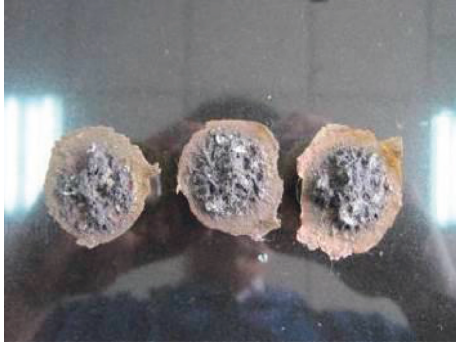
FIGURE 2: Fracture interface in pull-off test (70°C).
