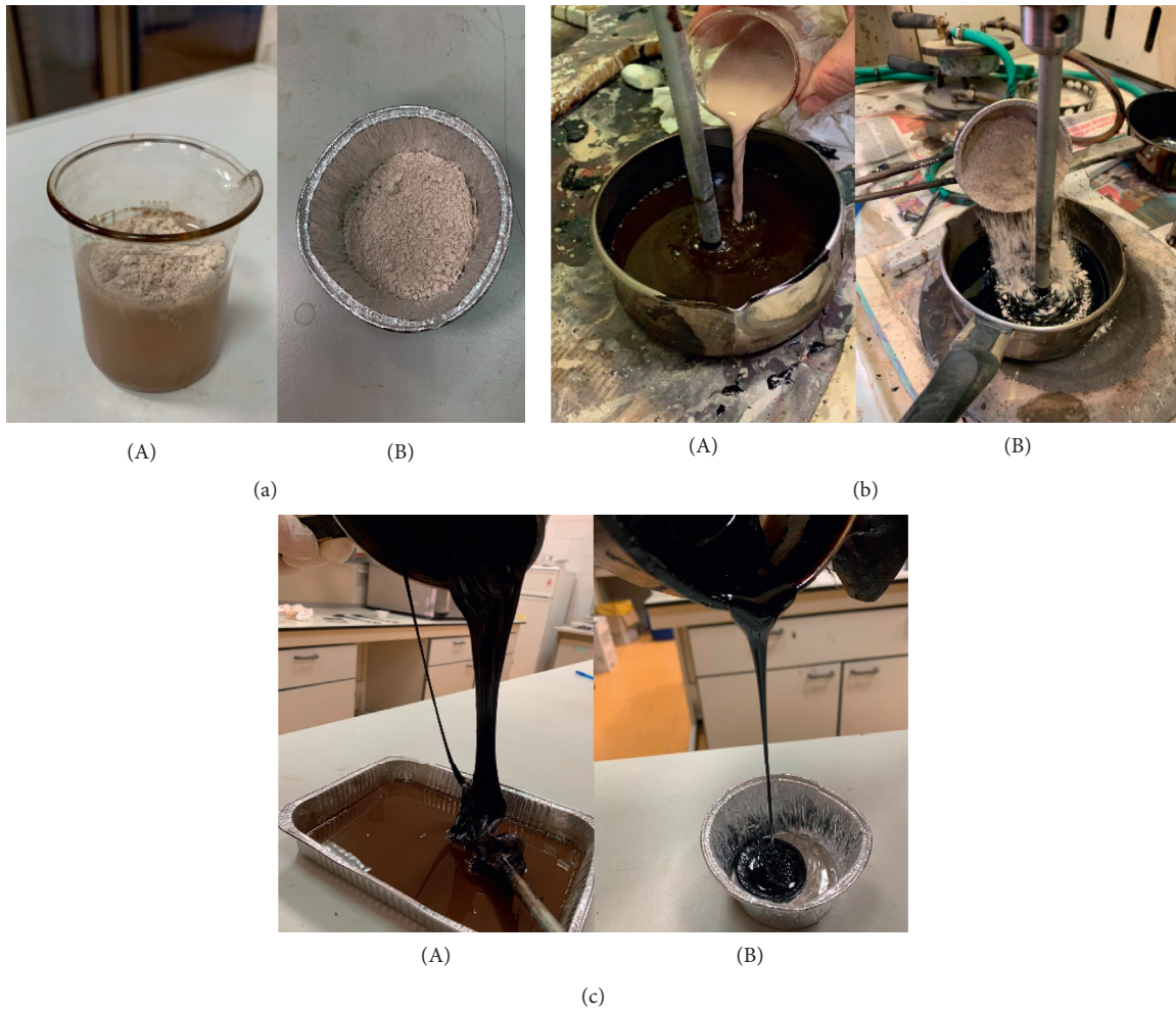
FIGURE 3: Mastic preparation using jet grouting waste. (a) Filler preparation: (A) cold mastic and (B) hot mastic. (b) Adding filler to the binder: (A) cold mastic and (B) hot mastic. (c) Final mastic: (A) cold mastic and (B) hot mastic.
