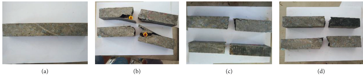
FIGURE 14: Fracturing behaviors of beam specimens of resin composite overlay reinforced with different fibers at 15°C. (a) Blank. (b) CF. (c) GF. (d) BF.
