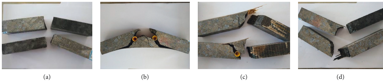
FIGURE 17: Fracturing behaviors of the beam specimens of resin composite overlays reinforced with different fibers at -10^{\circ}\text{C} . (a) Blank. (b) CF. (c) GF. (d) BF.
