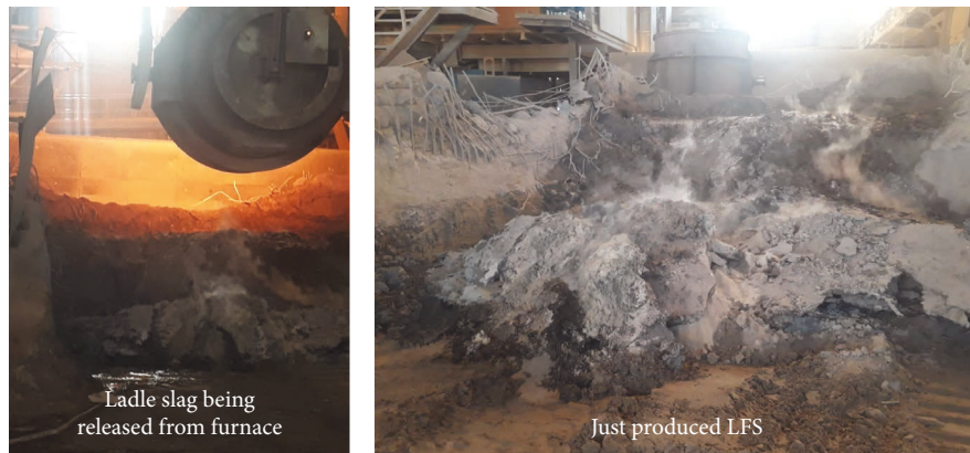
FIGURE 2: LFS as produced in Mirsarai plant of BSRM.
