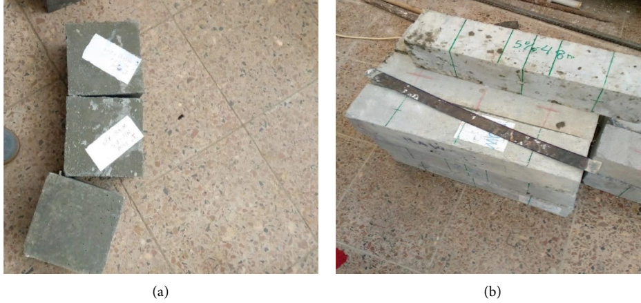
FIGURE 1: Test samples. (a) Cube specimens and (b) beam specimens.
