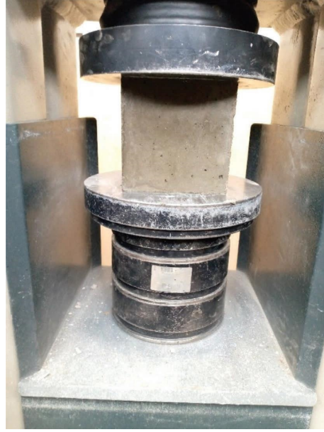
FIGURE 3: Compressive strength testing setup.
