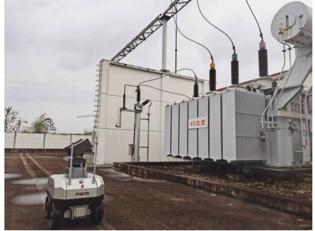
FIGURE 6: Process diagram of robot executing infrared temperature measurement task.
