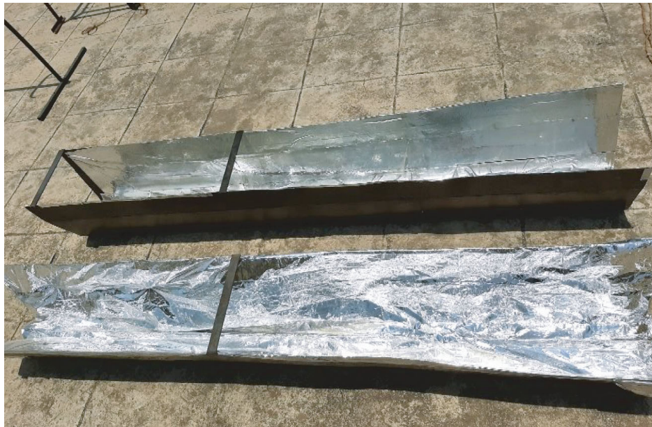
FIGURE 2: CPC with aluminum foil and chrome mirror silver vinyl wrap.
