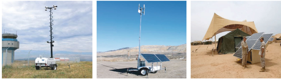
FIGURE 2: Solar remote power station [5].
