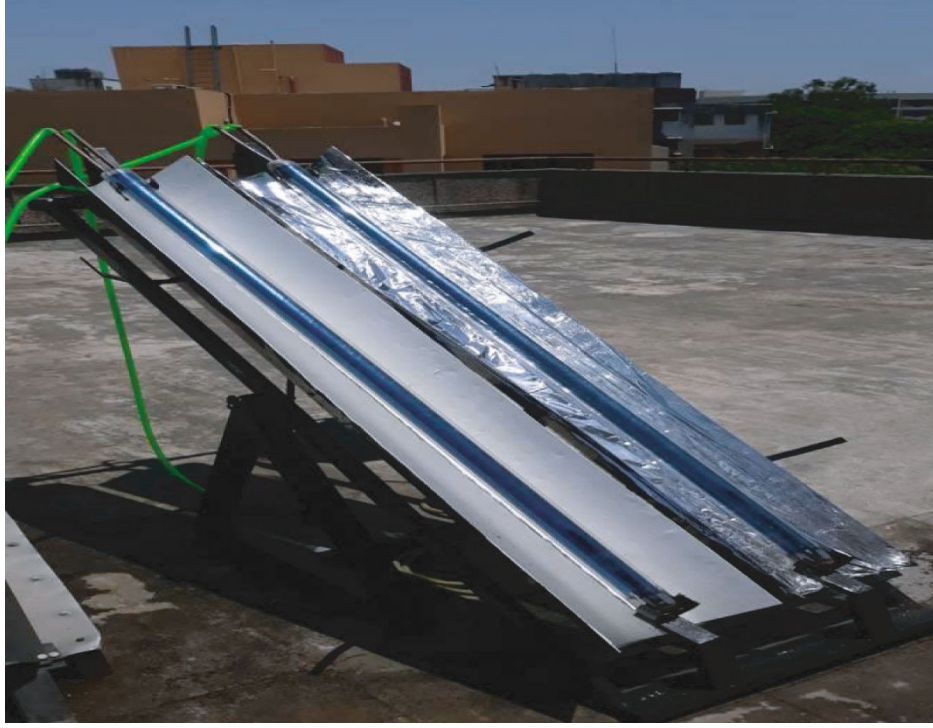
FIGURE 3: CPC with aluminum foil and Mylar.
