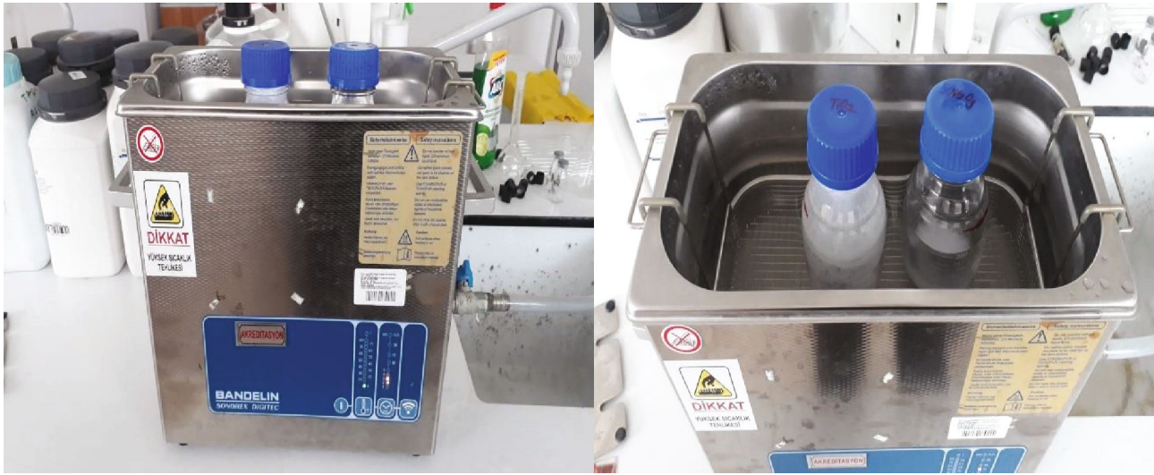
FIGURE 1: Ultrasonic bath setup.
